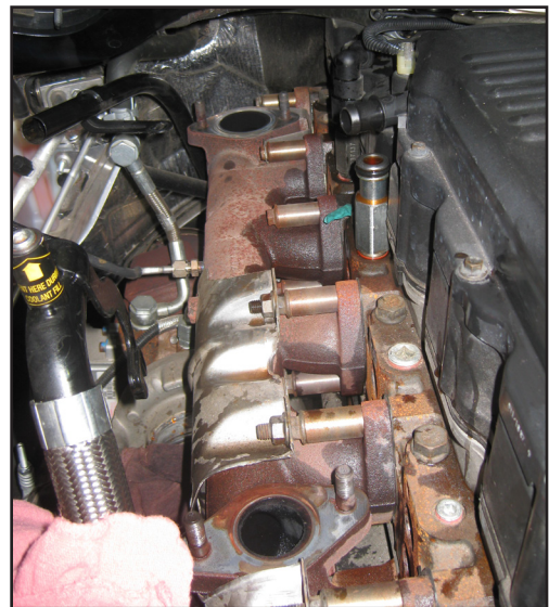
This is the “after” picture showing the EGR cooler assembly removed from the exhaust manifold.
