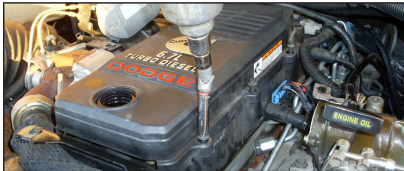
Removing the eight 8mm bolts that hold the CCV filter in place. DO NOT use the impact tool to reassemble and tighten the bolts.
