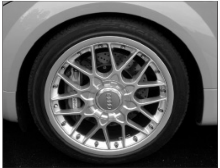
Figure 7 – Filling the wheel with brake hardware
